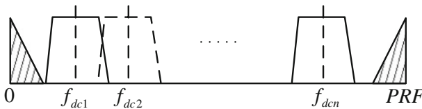
Fig. 2.6 Principle of the spectrum filtering algorithm
