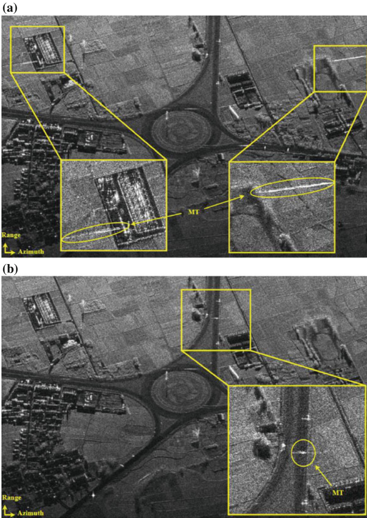
Fig. 3.16 Imaging results of the data without and with the proposed algorithm. a Stationary image of the scene without moving target imaging. b Imaging result of the moving target by the proposed algorithm
